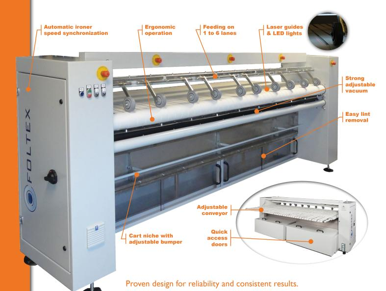
**FlexFeed SP** drastically improves productivity and quality by eliminating the need to manually stretch linen. The unit's internal vacuum keeps each piece of flatwork taut,
